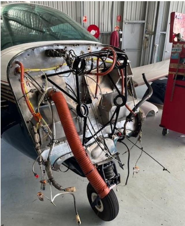
An engineless SJT with a clean firewall and engine support frame back in, minus the 4 shock mounts
