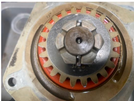
Correctly fitted elastomer coupling located in its cup
