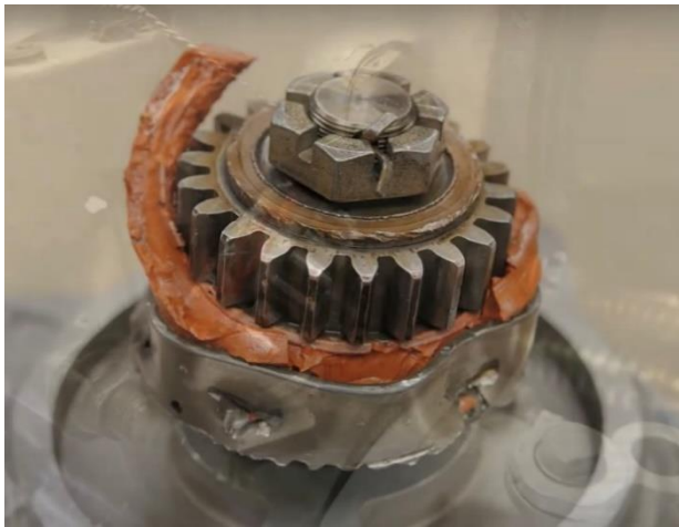
The elaborate drive gear into which the alternator coupling gear is engaged
