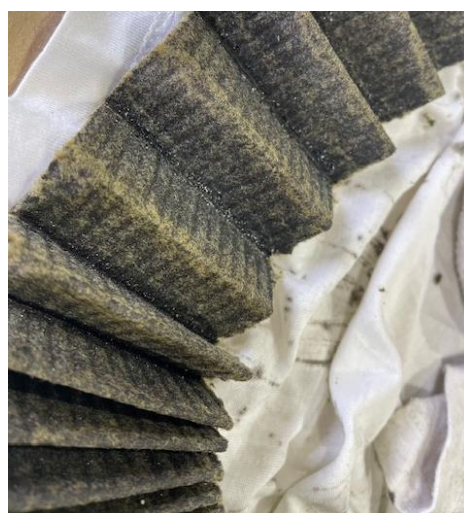
Oil Filter internals showing metal particles
