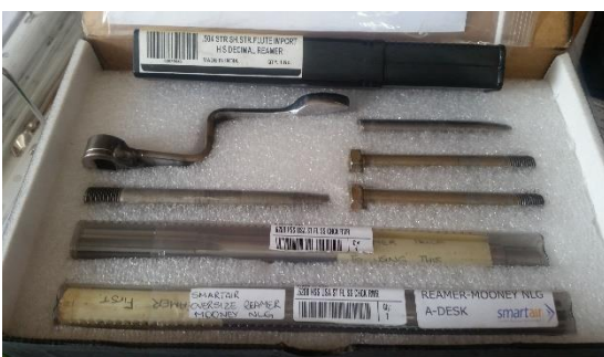
Prop Nut Removal Tool P/N MT002, Oversize Reamer NLG x 2 P/N KIT122R
