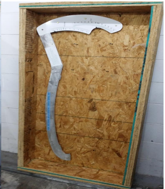
Aileron Travel Board 030003-200 ALL M20 Aircraft
