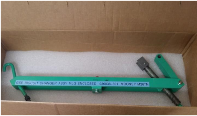
Shock Disc Tool MLG Enclosed M20TN P/N 030038-501
