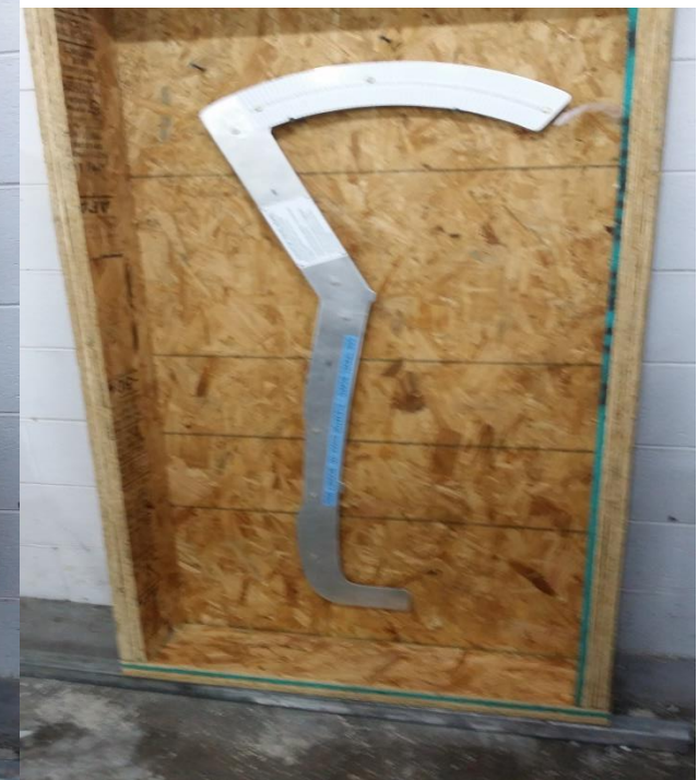
Elevator Travel Board 030004-100 M20C,D,E,F,G,J,& Mark22
